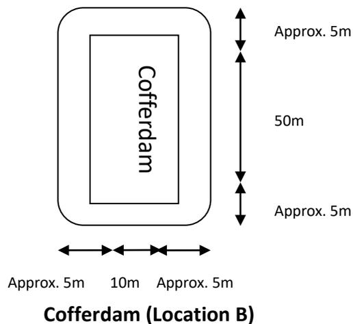
In these connections, the total lengths of silt curtains at Location A, B, and C were calculated, which were 50m, 160m, and 10m respectively.
