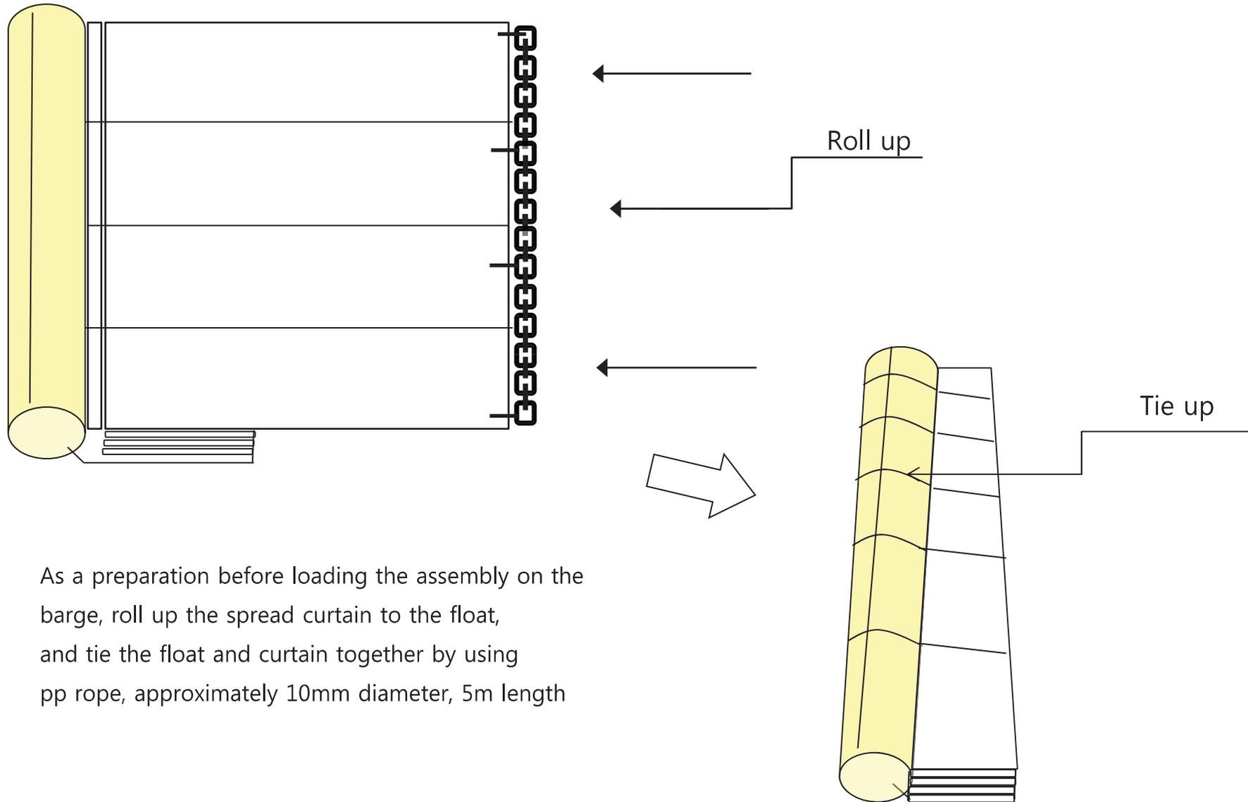
As a preparation before loading the assembly on the barge, roll up the spread curtain to the float, and tie the float and curtain together by using pp rope, approximately 10mm diameter, 5m length
