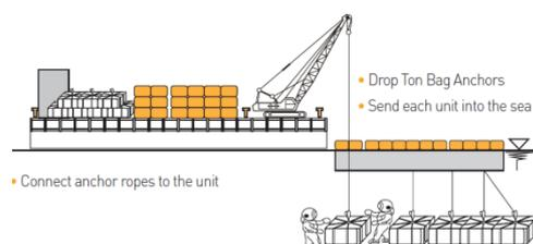
Deployment –Surveyor will help to set out the location of deployment. Ton Bag Anchors will be deployed on the seabed and silt curtain units will be unloaded in the sea. Then, diver / worker will connect the anchor ropes to the units (please refer to Appendix A for the connection details). Dive checking would be carried out to ensure the components were well installed in the right positions.
