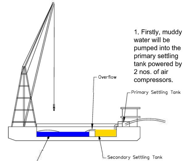
1. Firstly, muddy water will be pumped into the primary settling tank powered by 2 nos. of air compressors.
